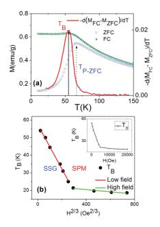
FIG. 5. (Color online) (a) ZFC/FC curve and the derivative d  $[M_{FC}-M_{ZFC}]/dT$  indicating peak temperature of  $M_{ZFC}(T_{pk})$  and mean blocking temperature  $(T_B)$ ; (b) Two straight AT-line fits for low- and high-field regime. (Inset) The evolution of blocking temperature  $(T_B)$  with measurement field.
