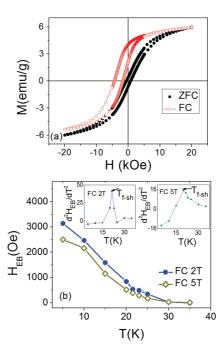
FIG. 7. (Color online) (a) *M*-*H* hysteresis loops at 5 K under FC (2T) and ZFC conditions; (b) temperature dependence of exchange bias field measured for cooling magnetic fields of 2 T and 5 T. Insets show the  $\frac{d^2 H_{\text{EB}}}{dT^2}$  vs. *T* curves for cooling magnetic fields of 2T and 5T.
