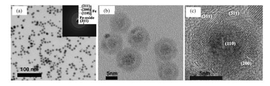
FIG. 1. Bright field (a) TEM and [(b) and (c)] HRTEM images of  $Fe/\gamma$ -Fe<sub>2</sub>O<sub>3</sub> core-shell nanoparticles. [Inset (a)] Selected area diffraction pattern.
