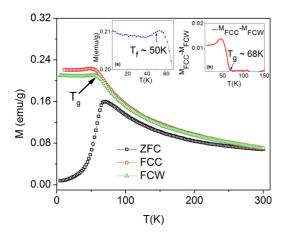
FIG. 2. (Color online) Temperature dependence of magnetization for zero-field cooling (ZFC), field cool cooling (FCC), and field cool warming (FCW). [Inset (a)] The dip in  $M_{\rm FCW}$  is associated with onset of spin freezing ( $T_f \sim 50$  K) and (b) shows the difference ( $M_{\rm FCC}$ - $M_{\rm FCW}$ ) plotted against temperature, where a sharp rise ( $T_g \sim 68$  K) marks the onset of thermal hysteresis.
