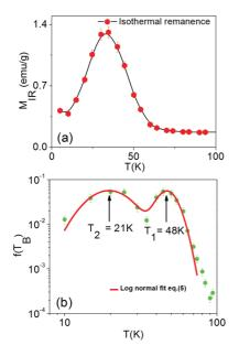
FIG. 6. (Color online) (a) Temperature dependence of isothermal remanence and (b) distribution function fit to Eq. (5).
